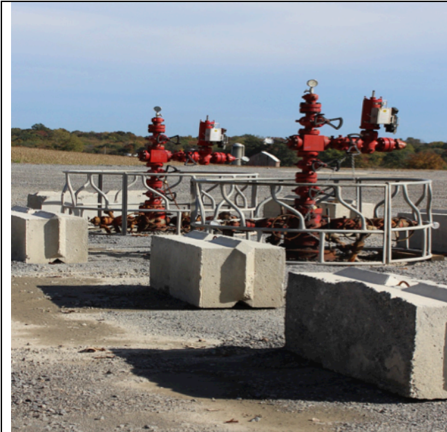
Figure 2 - Shell shale gas well pad after the well has been drilled. Pad sites are typically about the size of a soccer field.
